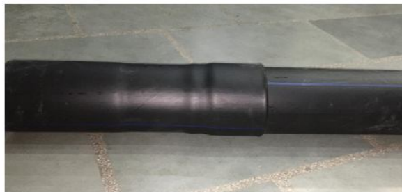
Photographs of HDPE Pipe with coupler arrangement
